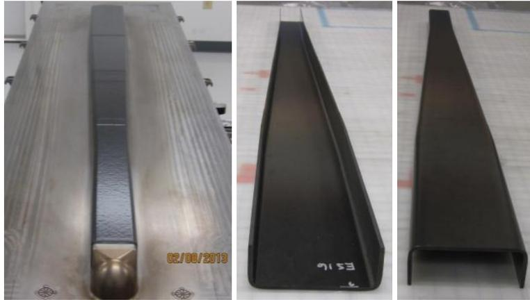
Figure 13. Tapered Spar on Tool After Final Debulk and After Cure
