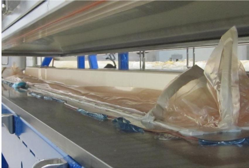
Figure 11. Bagged Spar Ready for Quickstep Cure
