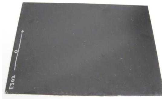
Figure 4. Representative epoxy panel cured using optimized cure cycle and bagging scheme
